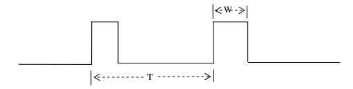
Note that the pulse width **W** is ranging from 1.0msec to 2.0msec. The period of the RC PWM pulse **T** is 40msec.
