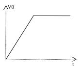
If the maximum acceleration of motor 0 is to be set at 2000mm/sec/sec, use the following code,
