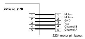
Note: Connecting the pins wrongly may results in damage of incremental encoder.
